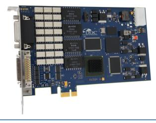
DDC's MIL-STD-1553 PCI-Express Card is designed with a one lane PCIe interface to be compatible with all PCIe slots in standard desktop computers. The combination of 1553 with digital and avionics Discrete I/Os offers flexibility that makes the card ideal for test applications.
