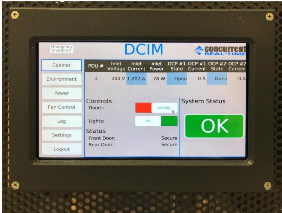
Figure 1. Cabinet Control Module display
